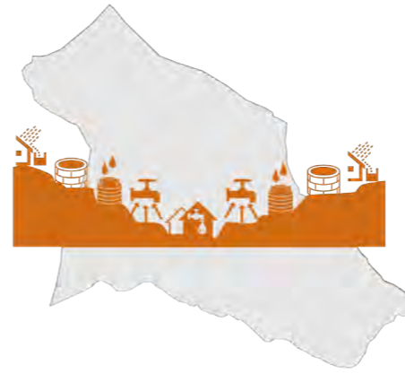
14. Piped water access at the bottom of the valley but shared water tanks and other self reliant water facilities higher up the valley.
