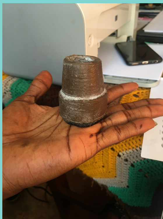
AT produced by MSL: PETs (left); replacement rubber tip for crutches (right). Photos: Nada Sallam
